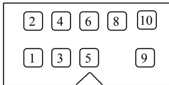
Pin 1 Power supply Pump : + 5VDC      **or**      + 12VDC
